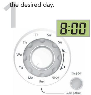
Spin the outer bezel to enter the desired wake time.
